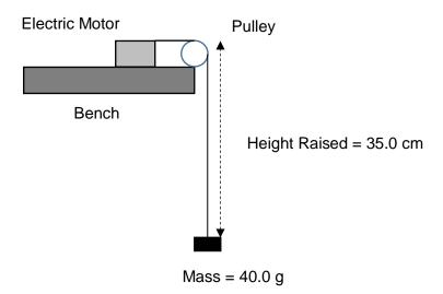
The students gradually increased the electric power provided to the motor by increasing the voltage on a power pack. They had performed an experiment prior to the investigation and determined that the average electric resistance of the motor was equal to 7.30  $\Omega$ . For each increased power, the average time for the mass to have its height increased by a distance of 35.0 cm was measured. The table below summarises the results obtained by the students.
